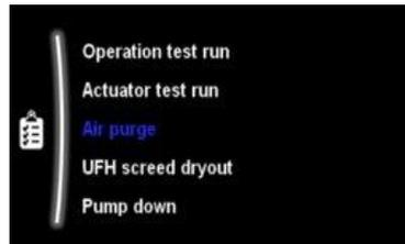
Figure 8: Daikin MMI Interface Air Purge Flow Rate Check Instructions. Image taken from Daikin Altherma 3 Monobloc User Interface Basics and Start-Up Guide
