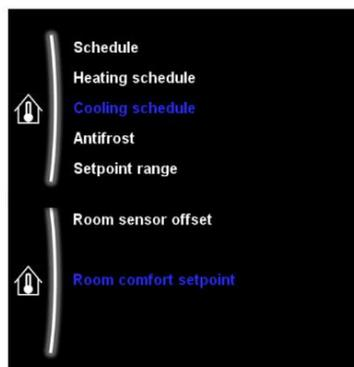
Figure 15: Daikin MMI Interface Room Settings. Image taken from Daikin Altherma 3 Monobloc User Interface Basics and Start-Up Guide
