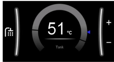
Figure 17: Daikin MMI Interface Tank Settings. Image taken from Daikin Altherma 3 Monobloc User Interface Basics and Start-Up Guide
