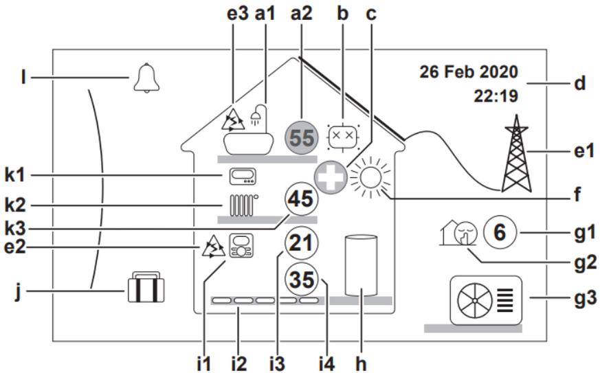
Figure 22: Daikin MMI Interface Possible Screens Key. Image taken from Daikin Altherma 3 Monobloc User Interface Basics and Start-Up Guide
