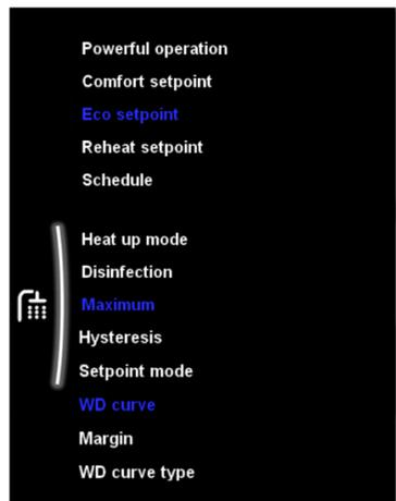
Figure 18: Daikin MMI Interface Tank Settings. Image taken from Daikin Altherma 3 Monobloc User Interface Basics and Start-Up Guide
