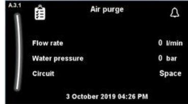
Figure 7: Daikin MMI Interface Air Purge Instructions. Image taken from Daikin Altherma 3 Monobloc User Interface Basics and Start-Up Guide (4)
