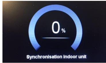
Figure 19: Daikin MMI Interface Synchronisation Screen. Image taken from Daikin Altherma 3 Monobloc User Interface Basics and Start-Up Guide
